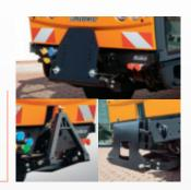
Equipped with a front-mounted quick-change system in the form of a coupling triangle or attachment plate (Multicar TREMO T: attachment plate with integrated lifting equipment and mechanical inclination adjustment)
